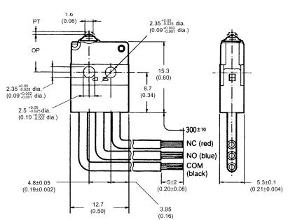
Note: 1. Unless otherwise specified, a tolerance of ±0.4 mm applies to all dimensions.
